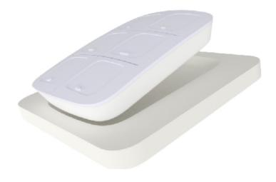
The Scene Selector can be used to control other smart home devices and is an essential part of any smart home. Utilizing Zigbee and a pairing button, the introduction of this device into a smart home is very easy. The Scene Selector has 6 buttons that can be individually configured.
