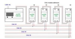
Each DALI port must have a unique I2C address set for the euLINK gateway to distinguish between them. Address setting is done by moving 2 sliders on the DIP switch, visible at the top of the DALI port board. Right next to the DIP switch is a multi-coloured LED that indicates the set address. The following 4 I2C addresses are possible:
