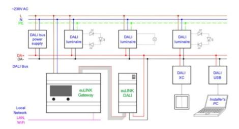
The installer's computer with the DALI programmer visible in the diagram should be used to address and group DALI luminaires and to carefully check the entire installation before integration with the euLINK gateway. If the DALI installation does not work properly, the integration will not improve this condition, and it is very possible that it will worsen it.
