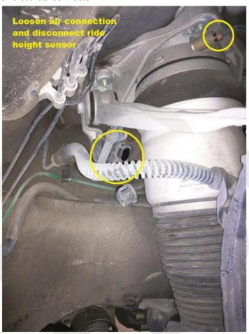
Undo the wires that run down the steering knuckle by wiggling their rubber grommets out of the corresponding brackets. Also unplug the connector into the lower part of the air strut. You're trying to free up slack so the steering knuckle can fall forward when your undo the top ball joint, as well as free the strut for removal.
