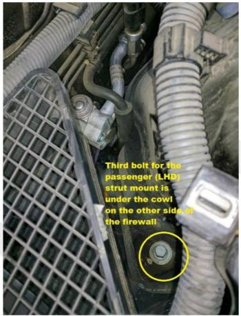
Using a 16mm or 5/8" socket on a long extension, remove two of the three bolts that hold the air strut mount. They shouldn't be terribly tight. I recommend removing the two bolts closest to the firewall (one on either side) – the remaining bolt (closest to the front of the car) is pretty obvious and easy to get a wrench/fingers on. The driver's side (LHD) looks like this:
