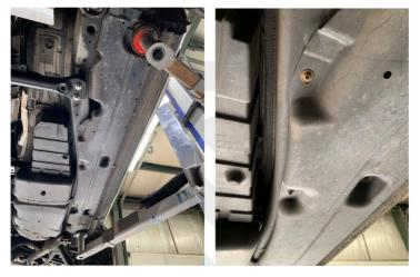
2. with the covers removed you will see all the body plugs that will need to be removed in order to install the rock. They are just snapped in so you can pop out by hand or with a flat head, there is 6 total, the other 2 arrows point to the mounting points that are already threaded in the body, and the other 2 smaller blind holes are for the smaller locking hardware.
