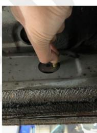
Next with the hand of a friend install the rock slider into One person guiding the holes to line up with the hardware you have installed. With the rock slider lined up and thread of the hardware sticking into the rock slider install the supplied nuts and washers onto the rock slider. At this point just install everything hand tight because you can make adjustments later and then torque them down.
