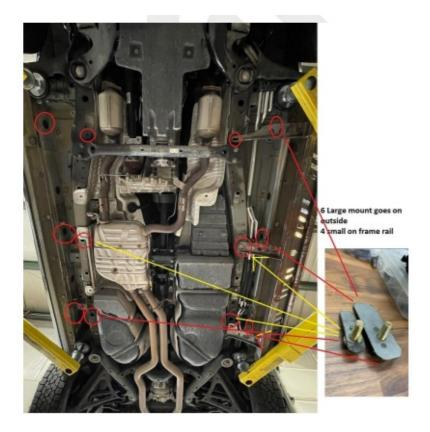
Guys with Air suspension follow these steps on the front brackets on both sides. Remove 13MM bolt on the factory frame and install longer supplied bolt on both sides. The air suspension rock sliders front mounting bracket is the only difference between setups.
