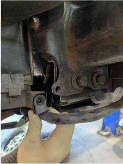
This is the TYPE B intercooler relocation that allows for even more clearance for bigger tires. Installation is same for both types.
