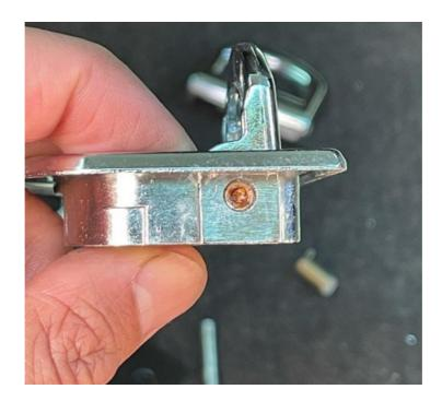
• Needs to be drilled out using 1/8 inch drillbit.
