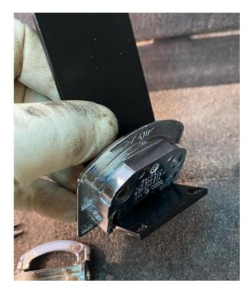
• Test fit it before bolting the rail system on to confirm it is clocked in the right position. Do not tighten it down as you will install the rails next.
