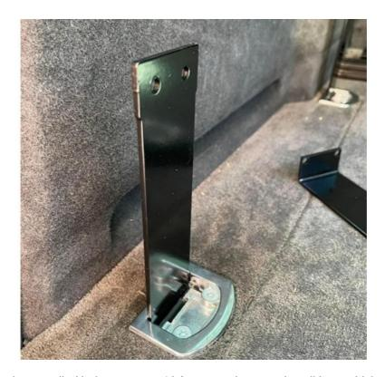
Now install the rails using supplied bolts torque to 10 foot pounds now reinstall into vehicle and reinstall the OEM Torx screws.
