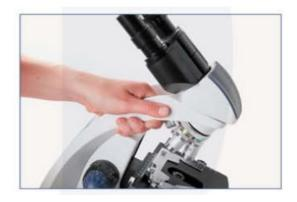
**Caution!** Hold the microscope at the top of the stand arm when it is moved. Holding the microscope by its stage or focusing knobs will damage the microscope
