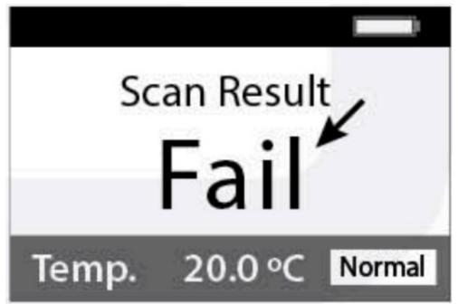
Out of calibration (zero sets) range Action: Make sure you are using the correct calibration solution, refer to the specification table. Make sure there is a sufficient amount of calibration liquid to cover the prism surface
