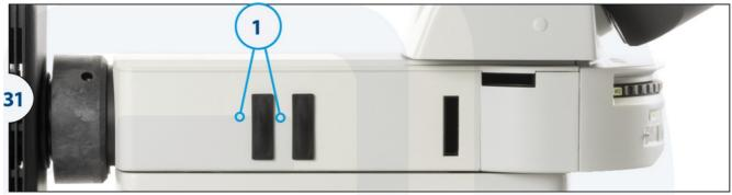
• "BF2" is the standard brightfield position. In case of high light intensity "BF1" can be used as it contains a neutral density filter to lower the light intensity
