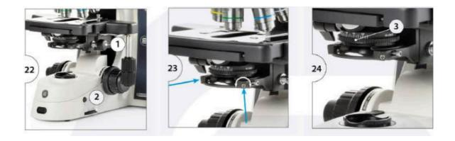
The aperture diaphragm (figure 24/3) should be used to adjust the numerical aperture, not to adjust image brightness. When the aperture diaphragm is opened to the  $70 \sim 80\%$  of objective aperture the ideal position is reached The simplest way to do this is to use the markings on the condenser
