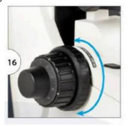
Next to the left side coarse focus know there is a ring setting the focus lock. The focus lock can be used to limit the maximum position of the stage at a certain height. This is ideal for preventing objectives to get damaged, slides from breaking or setting the stage at a reference height
