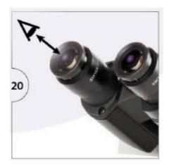
The eye point is the distance from the eyepiece to the user's pupil. To obtain the correct eyepoint, move the eyes towards the eyepieces until a sharp image is reached at a full field of view
