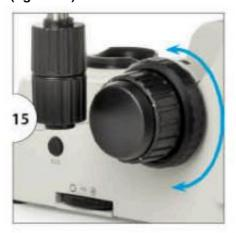
Next to the right side coarse focus know there is a ring for adjusting the coarse focus tensions. This can be used to make the coarse control move lighter or heavier, according to user preference
