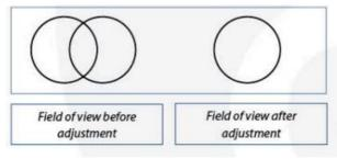
This distance can be set by either pulling the tubes towards each other or pulling them from each other. This distance is different for each observer and this should be set individually. When more users are working with the microscope it is recommended to remember your interpupillary distance for a quick setup during new microscopy sessions
