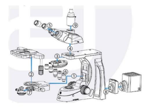
The diagram shows the order of each component's installation
