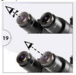
In order to compensate for human eye differences, distortion, thickness differences in cover glasses and tune for the best parfocality between objectives, one can use the dioptre to do so. Take a good prepared slide for your reference:
