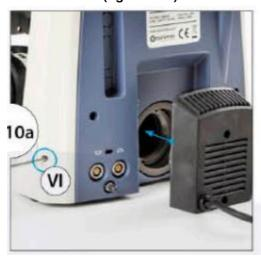
• Slide the lampunit (Halogen or LED) into position at back of the microscope base
