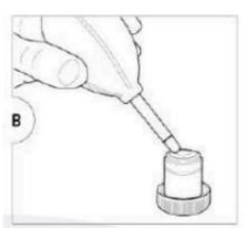
To prevent scratches on coatings and optical glass try to remove dirt and dust that sticks to the optical surface first with an air-blower or with pressurized dry air (oil-free and under moderate pressure version only)
