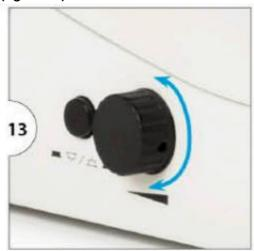
Next to the intensity controller, there is a button for switching between transmitted and reflected illumination. The standard brightfield configuration used for this manual does not have this option
