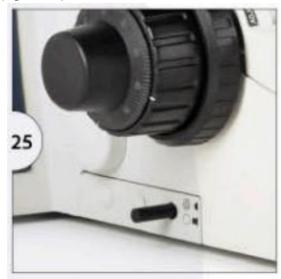
For LED models there is only 1 push button Push the button in for place the frosted filter into the light path
