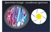
Aperture condenser set at 60% good contrast & resolution best resolving power
