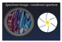
Aperture condenser set at 20% too contrasted image loss of resolving power
