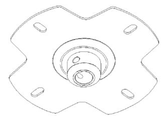
Insert the column into the ceiling plate and lock it into place utilizing the hexagonal wrench.
