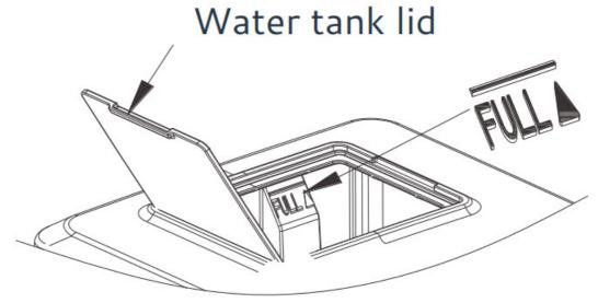
**Warning:** Do not pour water into the internal water tank located underneath the ice basket. This tank is not sufficient for proper ice-making.
