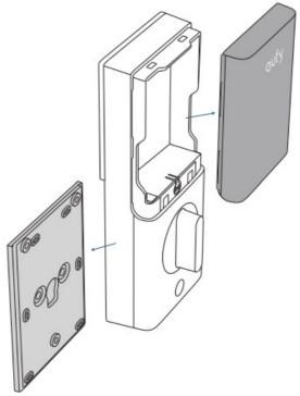
2. Run the cables through the slot on the mounting plate. Make sure the silicone pad is against the door.
