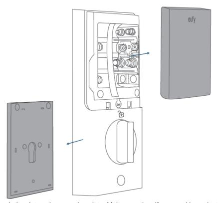
2. Run the cables through the slot on the mounting plate. Make sure the silicone pad is against the door.
