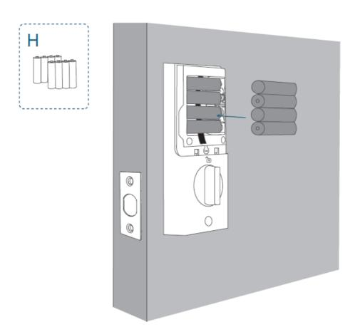
**Friendly Reminder:** When removing the batteries, first remove the upper layer, then gently pull the ribbon to lift the remaining batteries out of the compartment.
