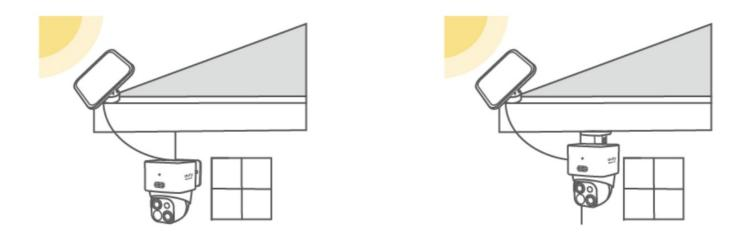
1. Drill holes with a 15/64 inch (5.95 mm) drill bit with the provided positioning card, then insert the anchors into the holes.
