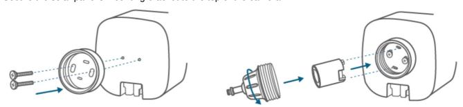
2. Install the solar panel onto the solar panel's mounting bracket by turning it.
