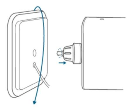
3. Connect the USB-C connector to the USB-C port of the solar panel.
