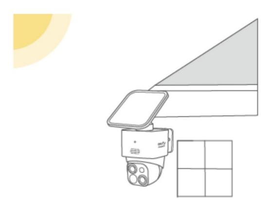
1. Secure the solar panel's mounting bracket to the top of the camera.
