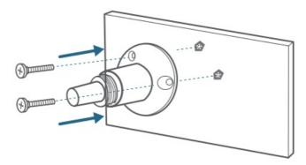
3. Firmly screw the knob of the mounting bracket into the mounting hole of SoloCam.
