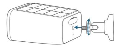
4. Hold and screw SoloCam to the mounting bracket. Rotate SoloCam to adjust the view and check it using the live stream which you can access in the eufy Security app.
