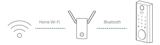
It can also work with the Battery-Powered Video Doorbell. For users who need an extra doorbell chime at a further location in the house, they can connect the Wi-Fi Bridge to the same home Wi-Fi network. The Wi-Fi Bridge will chime simultaneously when a visitor is pressing the doorbell button at the front door.
