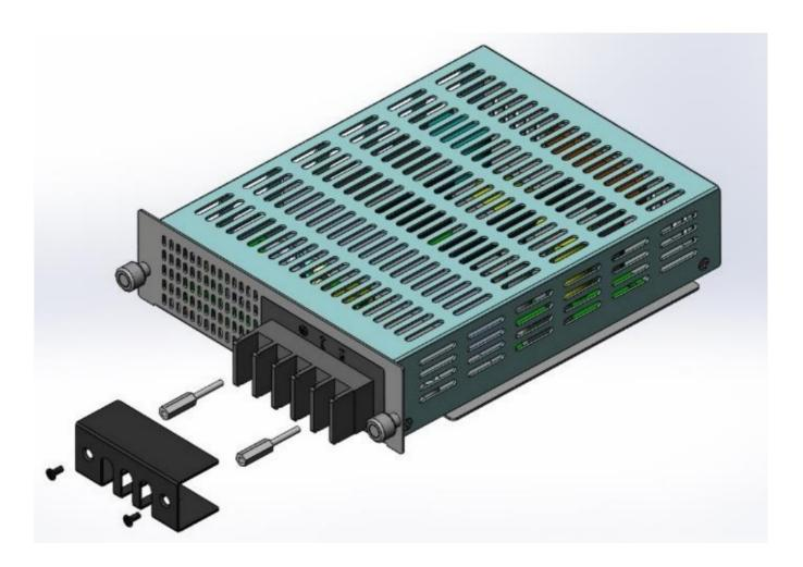
When stripping the cable sheath for connection to the terminal block, leave only 10mm of wires exposed for the connection.
