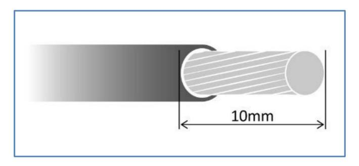
The power cord shall be IEC 60227 certified, rated 0.75 mm2 x 3C or UL recognized minimum 18AWG.
