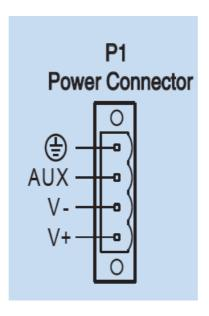
**NOTE:** When using the optional auxiliary power supply, the main power must be applied prior to the auxiliary power.
