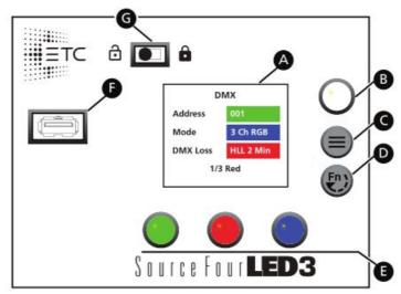
**A. Display**: The colors of options on the display correspond to the colors of the encoders below the display (E) and the Intensity encoder to the right of the display (B).
