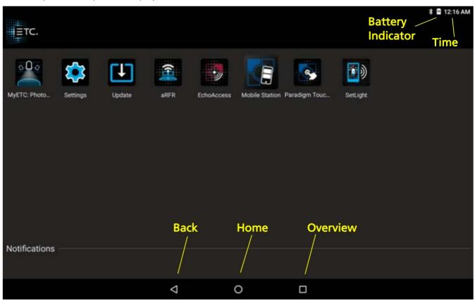
The home screen displays the icons for any ETC applications installed, settings for the ETCpad, and application update. Any notifications will display near the bottom of the display.
