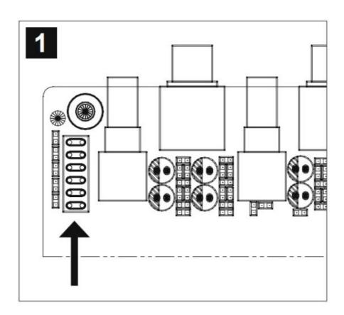
First, disconnect the device from the power supply. Then remove the housing cover and locate the six jumpers on
