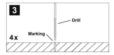
Lay the device aside and then drill the holes for the mounting screws at the marked locations. Please ensure not to damage any components of the vehicle while you drilling the holes. Alternatively (depending on the material of the surface) you can also use self-tapping crews.
