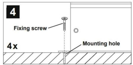
Then uphold the device to the chosen position and fix the screws through the mounting holes into the drilled screw holes.
