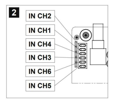
Then carefully remove the jumper on the desired input channel to set it to an input sensitivity of  $2 \sim 15$  V. Use suitable pliers for this.
