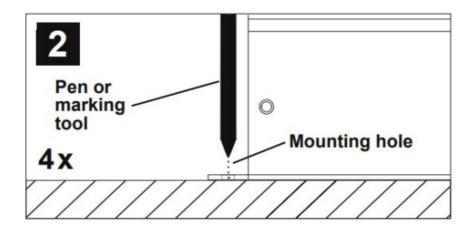
Keep the device at the chosen mounting location in the vehicle. Then mark the four drill holes with an appropriate
