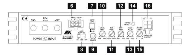
**6** Connect the INPUT RCA jacks of the included wire harness with the head unit by using appropriate audio signal cables. Make sure that the INPUT LEVEL push button (# 7) is in a LOW position (not pushed)
