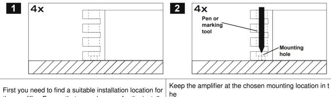
First you need to find a suitable installation location for the amplifier. Ensure that enough space for the installa tion of the cables remains and that they will not be ben t and have sufficient pull relief.
