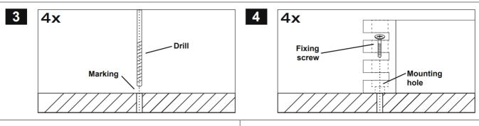
Lay the amplifier aside and then drill the holes for the mounting screws at the marked locations. Please ensure not to damage any components of the vehicle while you drilling the holes. Alternatively (depending on the material of the surface) you can also use self-tapping screws.
