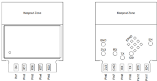
Figure 1: Pin Layout (Top View)
