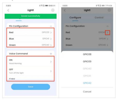
3. In the Configure tab, you may also customize commands to turn on or off the light and change its color. For example, you can set "good morning" as the command to turn on the light. Click Save to return to the previous screen. Then click Save again as shown below.
