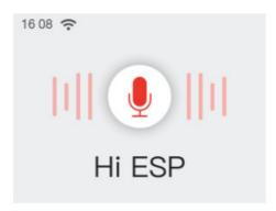
2. Utter a command within 6 seconds after the beep, such as "turn on the light". You will see the command shown on the screen and the LED light on the module turned on, and hear "OK". Around 6 seconds later you will exit the voice control screen if there is no more command.
