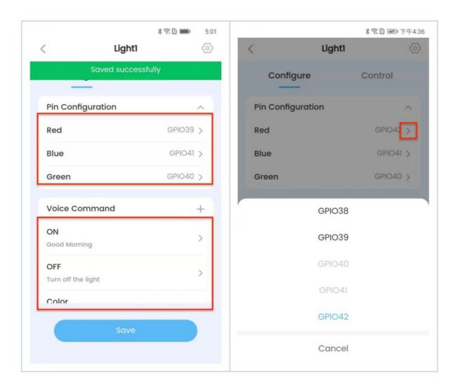
2.3 In the Configure tab, you may also customize commands to turn on or off the light and change its color. For example, you can set "good morning" as the command to turn on the light. Click Save to return to the previous screen. Then click Save again as shown below.
