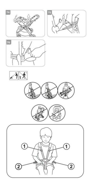
**ATTENTION!** Correctly mounted shoulder straps (1) should be located slightly above the child's shoulders, and the hip straps (2) should tightly hold the child's pelvis.
