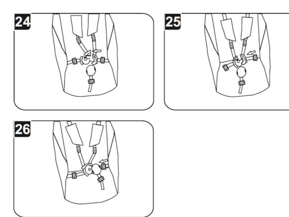
Check if the buckle is properly locked in place.
