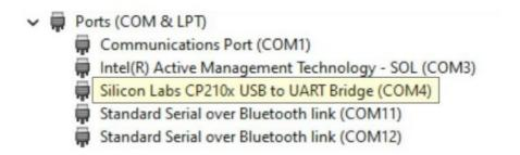
When using the espBerry, look for the Silicon Labs CP210x USB to UART Bridge. In our setup it shows COM4.
