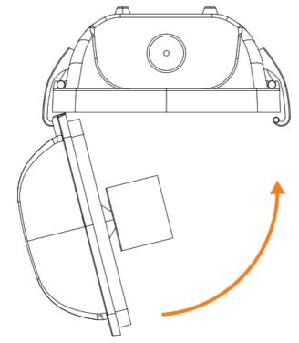
8. Secure lens to housing by locking the latches.
