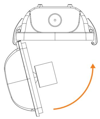
7. Secure lens to housing by locking the latches.
