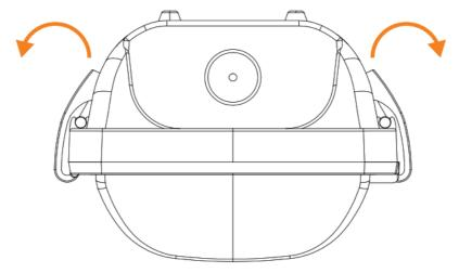
4. Without touching the LED boards, detach the LED tray and lens from the fixture.
