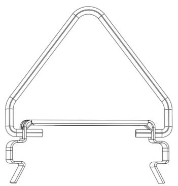
2. Secure the mounting clips to the housing recesses by firmly pressing them into place until both sides are secure.
