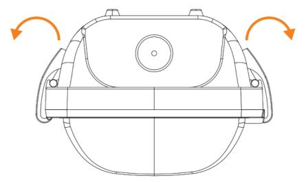
5. Without touching the LED boards, detach the LED tray and lens from the fixture.
