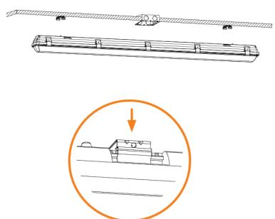
3. Release the latches by pulling the top away from the housing.
