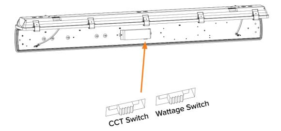
Select desired color temperature and wattage output combination with the switches located on the side of the driver.
