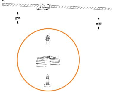
2. Fix the mounting clips to the housing recesses by firmly pressing them into place until both sides of the clip are secured.
