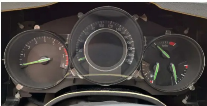
The instrument cluster attached with cable ties
