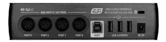
The rear panel features MIDI ports number 5 to 8, next to the USB **HOST** connector which is used to connect M4U eX to a computer. Right of it are the 3 **USB 3.0 PORTS** that allow you to connect and use any other USB device with your computer (i.e. USB keyboard, USB memory, USB dongle, etc.) and a **DC 5V** connector to connect M4U eX to the included power supply. To the very right top there is a standard laptop lock connector that you could use to prevent the unit from being stolen.
