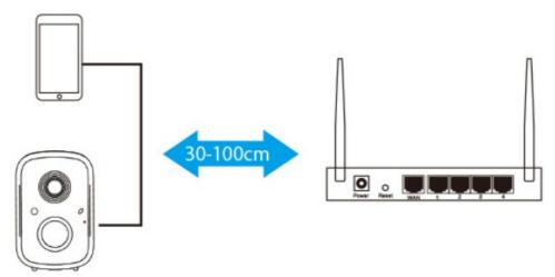
2. After the battery camera is powered on, there is a voice prompt "start match code" and the red LED light flashes. (Otherwise please press the RESET button on the camera for 8 seconds, it will be available after the voice prompt "reset successfully").
