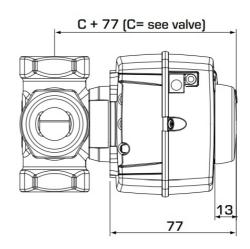
Installation dimensions for Controller Series CRC110 with ESBE VRG100, VRG200, VRG300, VRH100 and VRB100 mixing valves
