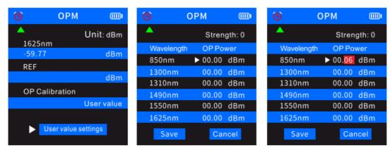
7. Select REF (Reference value), then press and hold the OK button (7) to save the current optical power value in the first blue line. The measurement unit will be switched to dB and cannot be changed to other units
