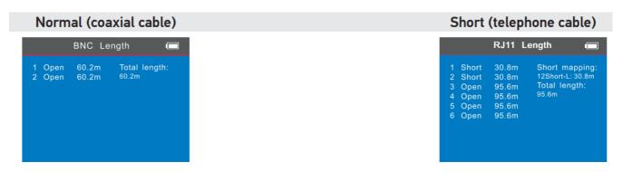
If the results for each pin differ noticeably, consider the result for pin 3 to be the reference value for the network cable length (the pin 4 result for a telephone cable and the pin 2 result for a coaxial cable respectively).
