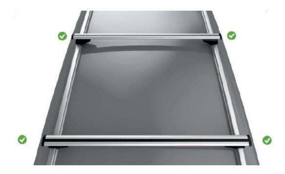
To check the fitment, firmly grasp load bars and attempt to move forward and backward, side to side.
