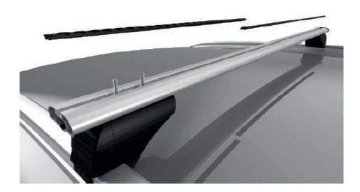
Take the rubbers off and insert T-Bolts. Insert the rubbers again after you remove T-Bolts.
