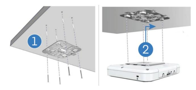
At the installation location on the ceiling, use the metal mounting bracket as a guide to mark four holes for the anchors and screws (included in the box). The mounting bracket is not intended for use with drop ceiling T-bars.
