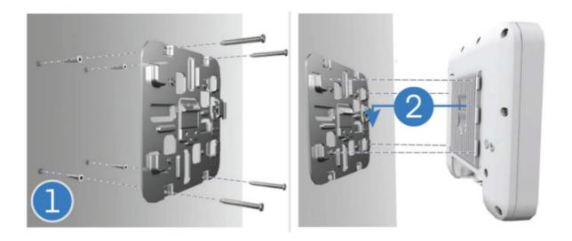
At the installation location on the wall, use the metal mounting bracket as a guide to
