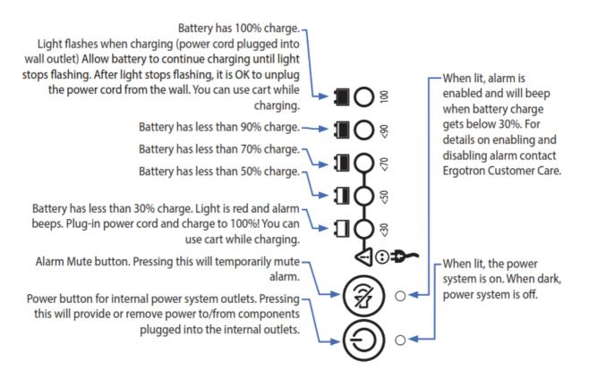
**NOTE:** Frequent operation of the cart while battery charge levels are below 30% will significantly reduce the life of your battery.
