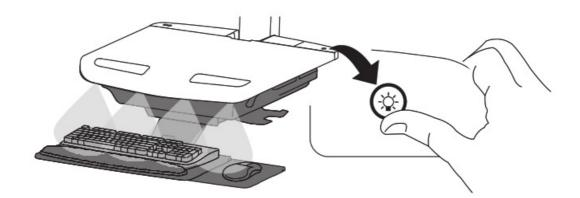
This power system interface will alert you to the percentage of charge remaining in the cart battery with a series of steady or flashing red, yellow, or green lights, and an alarm that will beep when the charge gets below 30%. Remember, the battery needs to be charged to 100% every day, and you can use the cart while charging, so plug in the cord as often as possible to avoid running out of power!
