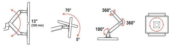
Caution: Leave enough slack in cable to allow full range of motion. "~ To avoid the potential to pinch cables it is important to follow the cable routing instructions in this manual. Falure to follow these instructions may result in equipment damage or personal injury.
