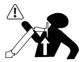
**WARNING!** Stored Energy Hazard: The arm mechanism is under tension and will move up rapidly, on its own, as soon as attached equipment is removed. For this reason, DO NOT remove equipment unless the arm has been moved to the highest postion! Failure to follow this instruction may result in serious personal injury andlor equipment damage!
