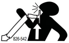
**WARNING!** Stored Energy Hazard: The arm mechanism is under tension and will move up rapidly, on its own, as soon as the attached equipment is removed. For this reason, DO NOT remove equipment unless the arm has been moved to the highest position! Failure to follow this instruction may result in serious personal injury and/or equipment damage!
