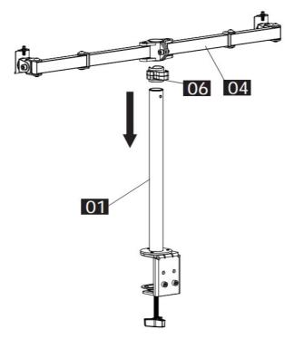
**STEP 2-2** Secure monitor connector [04] to the pole [01] then attach the cable clips [07] to the monitor connector [04]
