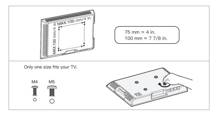
Bolt length: Verify adequate thread engagement with bolts or bolts/spacers combination. We recommend thread engagement by at least 5 turns.
