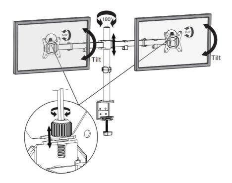
Individual VESA plate height adjustment helps monitors to be perfectly aligned.
