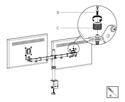
**STEP 6 Fix Tilt Angle of the Monitors**
