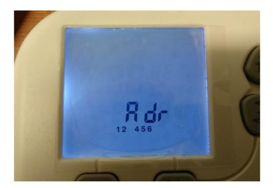
After a few seconds, the thermostat will return to the main screen. Plug in the receiver, and get the thermostat to resend the signal by turning it to a low temperature, waiting 30 seconds, and turning it to a high temperature. The receiver will switch on. If it doesn't switch on, there may be interference, please start again trying a new code.
