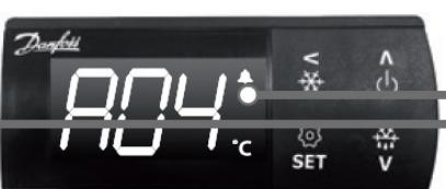
Temperature and alarm codes alternate flashes until the alarm resolved. The alarm bell is shown.
