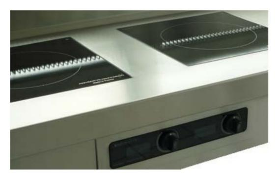
The cutout dimension for the separate control panel is 14-5/8" x 2-7/8". Maximum distance from the base unit is determined by the length of the included ribbon cable. Mounting is slightly different, as six 6 mm (15/64") holes will need to be drilled for the mounting bolts to pass through the countertop. NSF approved high temperature sealant is still required. Attach the nuts and connect the ribbon cable to the base unit.
