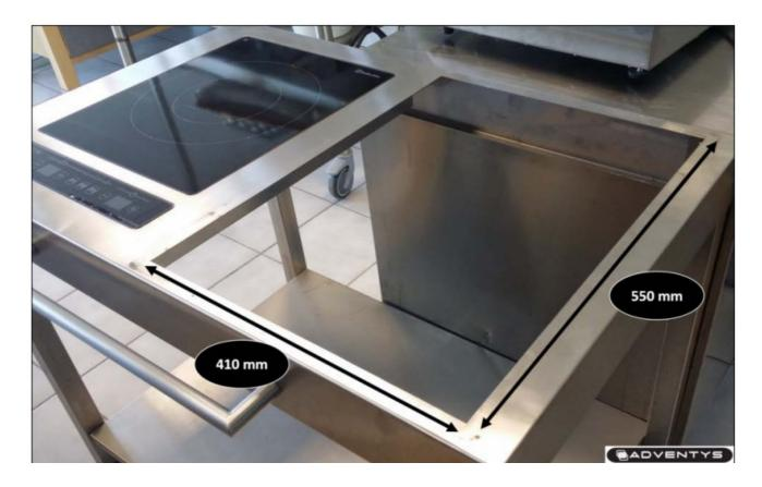
Dimensions of the unit are 17-1/2" x 23". The height is 6-3/4". Dimensions of the cut out need to be: 410 mm (16-1/4)" x 550 mm (21-3/4)".
