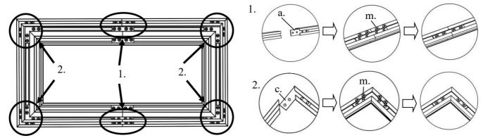
**Step 11:** Install the angle cover (n.) on each corner of the frame using the double-sided tape.
