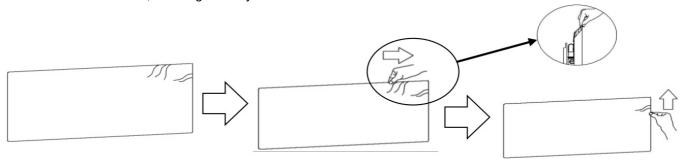
Incorrect material installation –The corners of the screen material are not properly wrapped along the edge of the frame leaving the material with unbalanced tension and an uneven finish. To correct, detach springs from material at the corner(s) where material does not lie flat along the edge of the frame, reposition the material so that it lies flat
