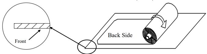
**Step 7:** Carefully and gently place the assembled frame on top of the screen material in the marked areas as shown below. Make sure to not allow the angle edge of the frame to come in direct contact with the screen material to avoid puncturing it.
