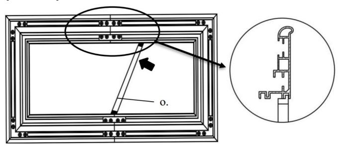
Step 9: Hook one end of the spring and secure inside the groove of the frame, use the spring hook (i) to attach the spring to the hole located on the screen material's outer edge in the following order.
