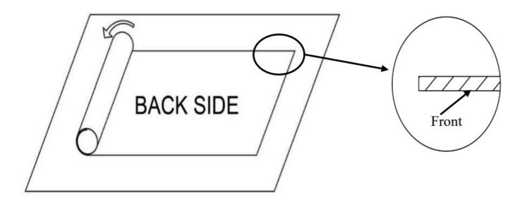
Step7: Carefully place the screen on top of the assembled frame as shown below.
