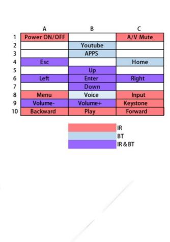
**Note:** IR always sends infrared, BT sends Bluetooth in Bluetooth state, IR&BT works simultaneously in Bluetooth state under Bluetooth
