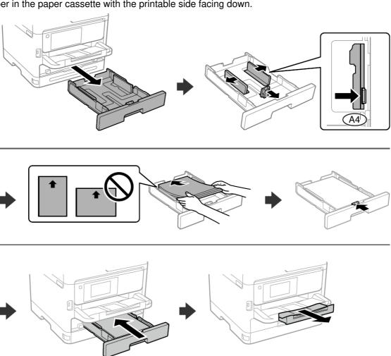
Do not load paper above the  $\ensuremath{\Downarrow}$  arrow mark inside the edge guide.
